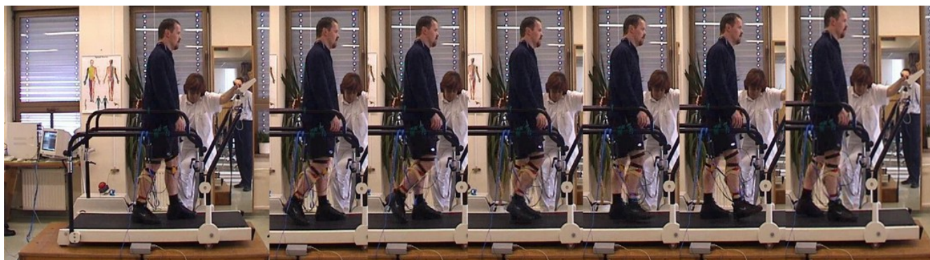
Fig. 3. Record of an incomplete SCI patient's walking with the peroneal electrical stimulation.
