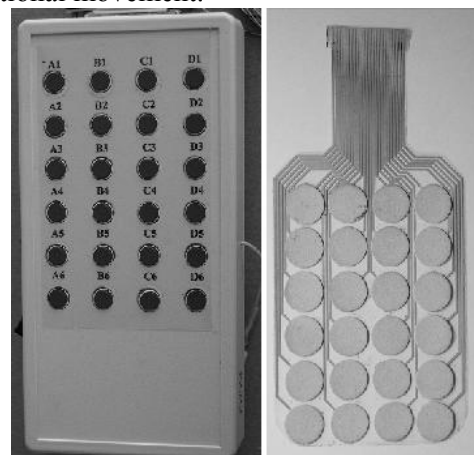
Fig. 1: Actitrode®: The 24-field electrode array (right) and the control box for selecting of the conductive fields (left).
