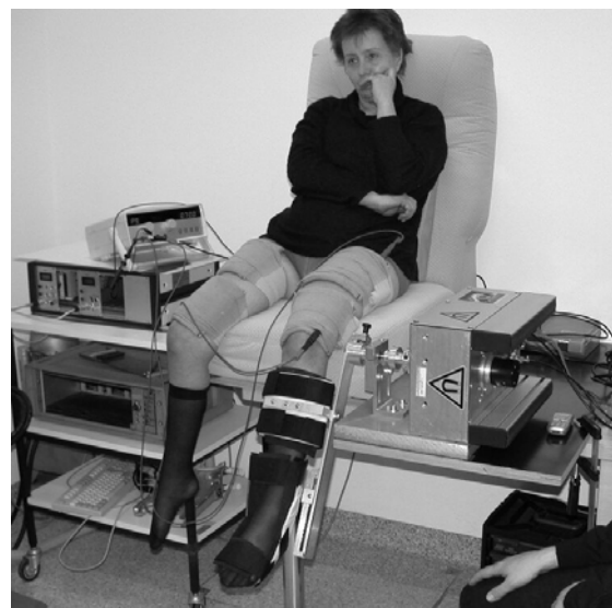
Fig. 1: Experimental setup with electrical stimulation and manipulandum connected to the lower leg.
