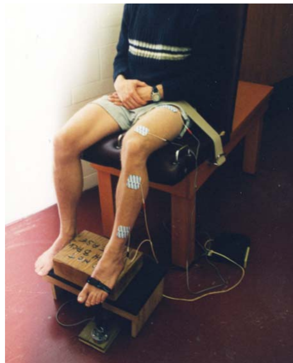
Fig. 1: Experimental setup for tibialis anterior force measurement. Electrodes placed for quadriceps and tibialis anterior stimulation. Load cell attached to floor.
