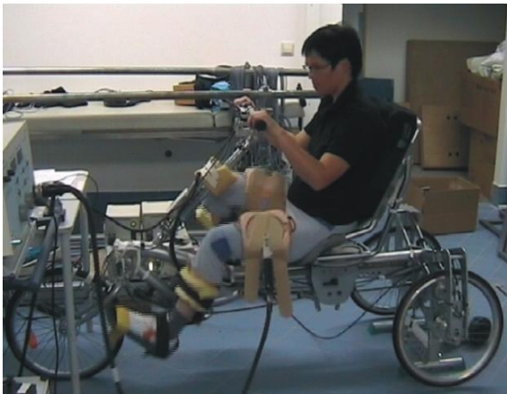
Fig.1. Stationary FMS-cycling (patient with complete SCI Th9). Left and right quad muscles stimulated by M&M PSTIM160 and MAGSTIM Rapid repetitive magnetic stimulators. Annular magnetic coils fixed by polystyrene-brackets were used.
