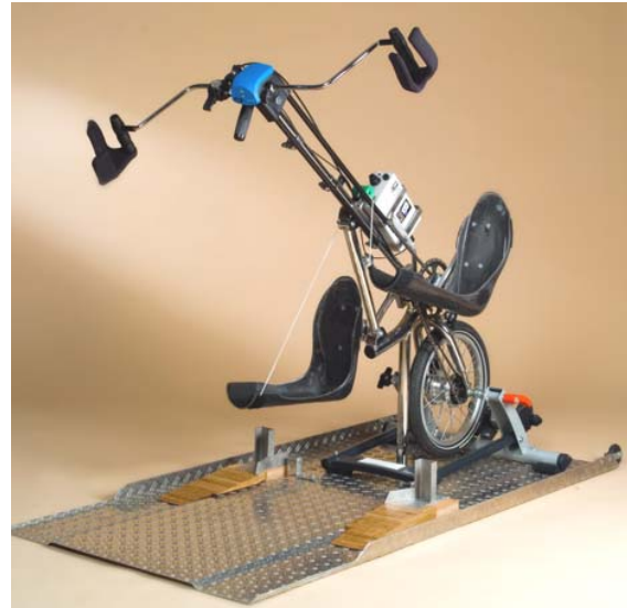
Photo 3: BerkelBike "Home" free standing system for SCI with a high lesion. White box is previous stimulator. Small blue box on the arm cranks is the controller for the Tacx software which has to be installed on a personal computer. The arm cranks are normally synchrone but in this example we tried asynchrone.
