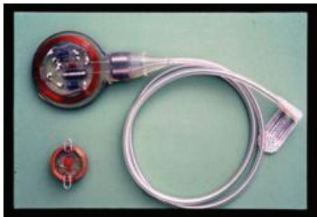
Fig 1: The Medtronic Peroneal Assist implantable stimulator and the Ljubljana JSI peroneal implant.
