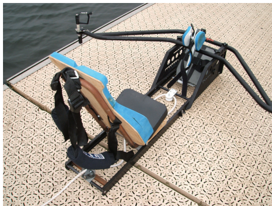
Fig 2(b) The Alden (16 & 18) detachable state room with modified seat, padded shoulder straps and bungee cord, pulley and cam cleat to allow adjustment of bungee cord tension. The telescopic leg stabiliser is similar to that used on the indoor rower.
