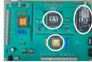
Fig. 6: Prototype of intraoperative stimulator (Stim3D)
