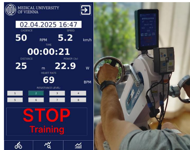
Figure 4: Left: Graphical User Interface to show realistic estimations of KPIs. It contains the current time with white background, the selection buttons for the resistance level, start and stop buttons to start and stop the training. KPI are cadence, speed, training time, distance, power and heart rate. Right: Hardware mounted onto the BerkelBike Fitness with the interface used during training.
