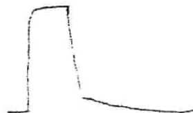
Tracing of 20 microsec. pulse
