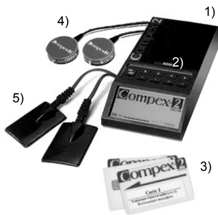
Figure 1: Compex Motion electric stimulator: 1) stimulator; 2) keypad with 9 push buttons; 3) three memory chip-cards; 4) two EMG sensors; and 5) two stimulation electrodes
