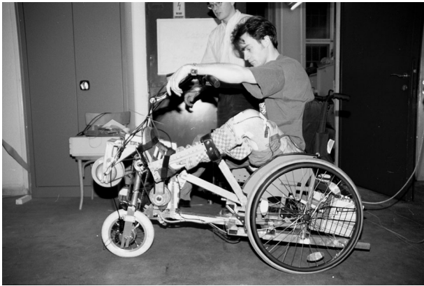
Figure 4: Paraplegic test person on the moving tricycle and results of measurements during steady-state cycling at crank angular velocity 33rpm. The results are compared to results of a simulation study /5/.
