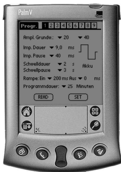
Fig. 2: PDA with developed software for programming the stimulator
