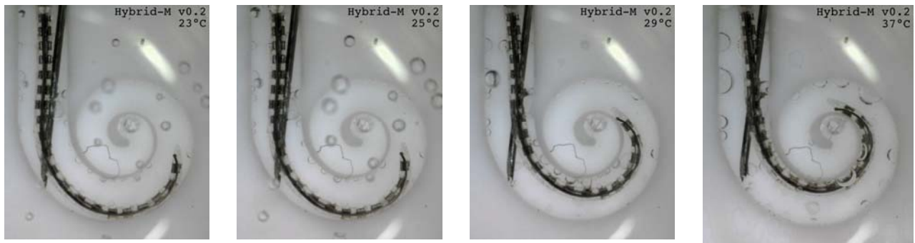
Image 1) Thermal characterization and intracochlear deformation behavior of the hybrid-M v0.2 (prototype electrode). Successive heating (20°-45°) was applied in a water bath. A substantial curvature at the tip is visible at 23 °C. However, the desired intracochlear movement of the electrode from the outer wall to the inner wall has been reached at 37°C. In addition to the positioning of the electrode in close proximity to the nerve cells in the central axis (modiolus) of the cochlea, the insertion depth is increased as a side effect by the activation of the shape memory effect.
