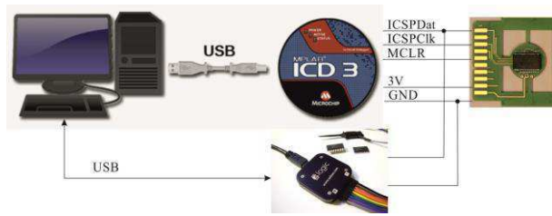
Fig. 2: Setup for calibrating the implantable stimulator Components: PC with Microsoft Visual Studio program for semi-automated testing, Microchip ICD3 flashing device, Salea Logic 8 Logic analyzer
