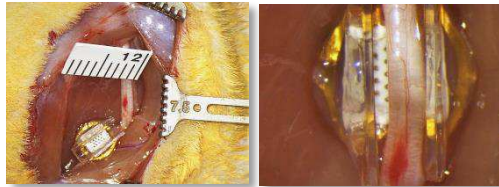
Figure 3a. WFMA devices mounted to silicone cuff used in Rat sciatic nerve implantation. Left: next to nerve, Right: implanted
