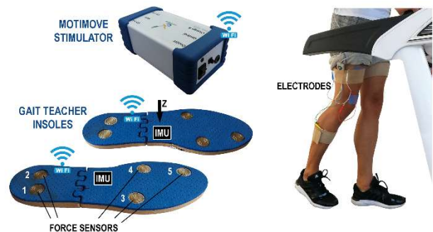
Fig. 1: “Gait teacher” with five robust pressure sensors and one 6D inertial measurement unit (left panel) and “MOTIMOVE” eight-channel stimulator to be applied via surface electrodes for the gait assistance in persons with hemiplegia.
