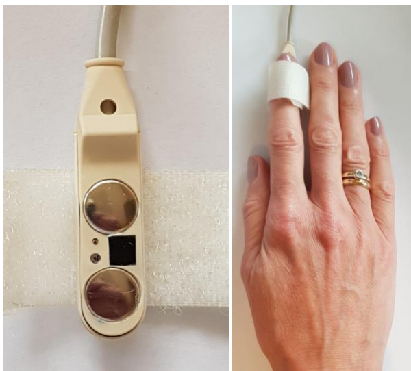
Fig. 1: Skin conductance measurement with finger sensor (Insight Instruments Hallein, Austria) (left) attached to the index finger of the right hand (right)
