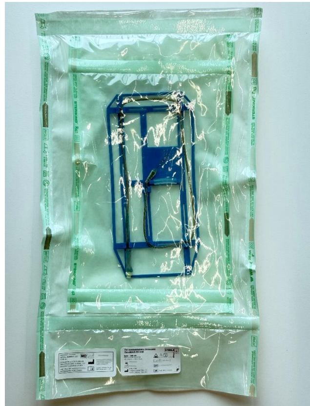
Figure 3: TIME implant manufactured, packaged and sterilized for an investigator-initiated clinical trial under ISO 13485 QMS. Labels contain required information according to regulatory needs. Transport and holding frame needed to be codeveloped for deployment.
