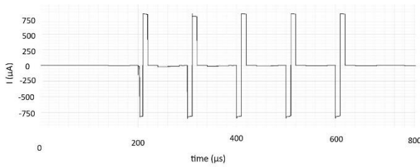
Figure 10: Output biphasic current for 10μs pulse width, 10KHz frequency and 820μA amplitude.
