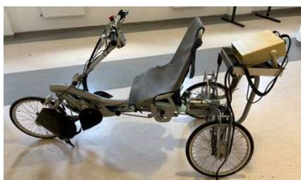
Figure 1: Special tricycle equipped with an electrical stimulator for SCI patients with denervated muscles
