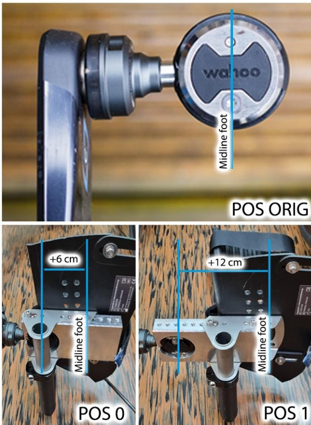
Figure 1: Mounting positions. Illustration of the different mounting positions. An adapter plate was used for mounting the ankle orthosis to the power pedals at different positions.
